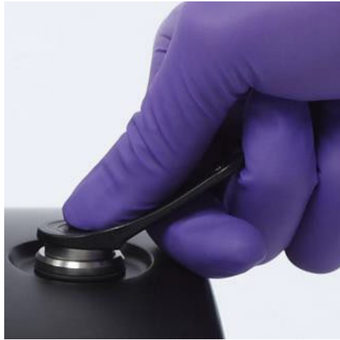
Figure 6-3 Holding Calibration Button to Button Reader
