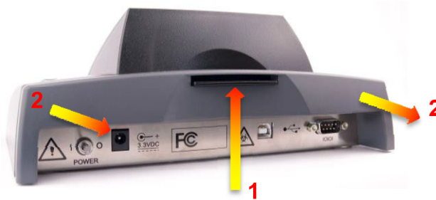
Figure 5-2 Remove Battery Holder Cover
