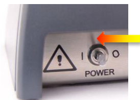
Figure 6-2 Turn Analyzer On
