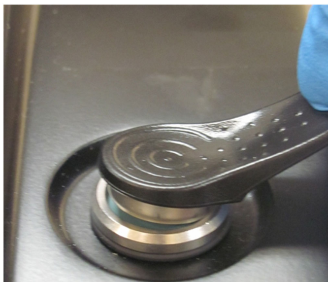
Figure B-6: Holding Calibration Button to Button Reader
