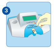
**Test:** Place a drop of sample on the sensor; results in 3 minutes.
