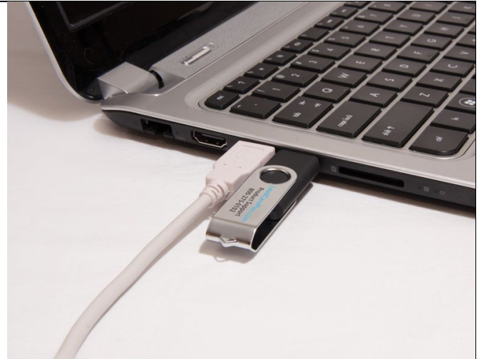
Figure 6-16 USB Cable and USB Memory Stick Inserted into USB Ports on PC
