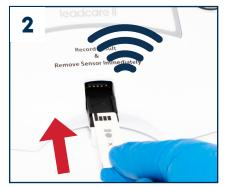
Insert the sensor (with black bars facing up) under the sensor guides on the sensor deck. Insert completely into the analyzer until you hear a beep.
