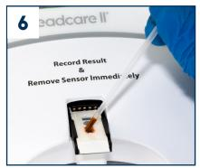
Touch the dropper tip to the X on the sensor and squeeze the walls to dispense the sample. The analyzer will "beep" and begin the 3 minute countdown.
