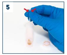
Remove the cap from the treatment reagent tube. Squeeze the walls of the dropper and insert into the sample. Release the pressure to draw some sample into the dropper.
