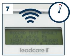
Wait 3 minutes until the test is done. The analyzer will beep and display the lead result in  $\mu$ g/dL Pb.
