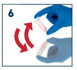
Replace the tube cap. Invert the tube 8 to 10 times to mix the sample completely. Control material in treatment reagent tube will appear red.
