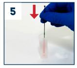
Place the capillary tube into the treatment reagent tube. Insert a plunger into the top of the capillary tube and push down, ensuring the entire volume of control is dispensed into the treatment reagent.
