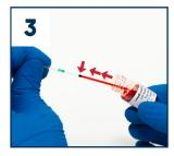
Holding the capillary tube almost horizontally with the green band on top, fill the tube to the 50  $\mu$ L black line. Replace the cap on the control vial.
