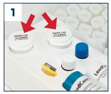
Remove a sensor from the sensor container. Close the container.
