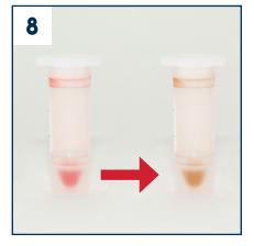
The sample is ready when the mixture turns brown. Samples may be stored up to one week if refrigerated.
