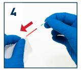
Wipe the outside of the capillary tube to remove any excess control.
