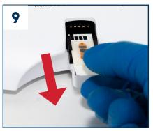
Remove the used sensor immediately after recording the test result.
