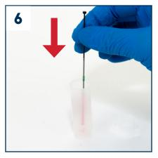
Place the capillary tube into the treatment reagent tube. Insert a plunger into the top of the capillary tube and push down, ensuring the entire volume of sample is dispensed into the treatment reagent.
